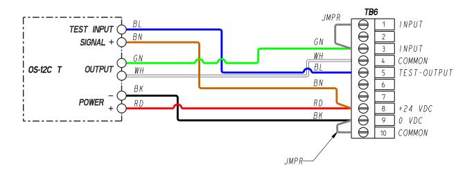
Program the OS-12 CT set to "**D**" - Active High / N.C. On the **iQ**: Set **INDEX** 20 to **VALUE 01** (Monitored Beam).
